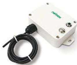
R718IA Wireless 0-5V ADC Sampling Interface
