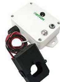
R718NL125 Wireless Light Sensor and 1-Phase Current Meter ( 1 x 250A Clamp-On CT )
