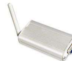
ZL01F IEEE 802.15.4 RS232 Straight-through Adapter
