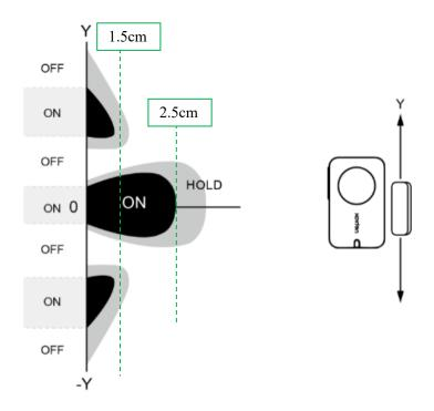
1. Tear off 3M release paper of the magnet body and attach the body to the door frame and stick it to the door in parallel with the door magnet body. (please do not stick it on the rough door to avoid falling off after using the device for a long time).
