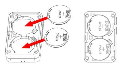
Note: To install the battery, use a screwdriver or similar tool to assist in opening the battery cover.
