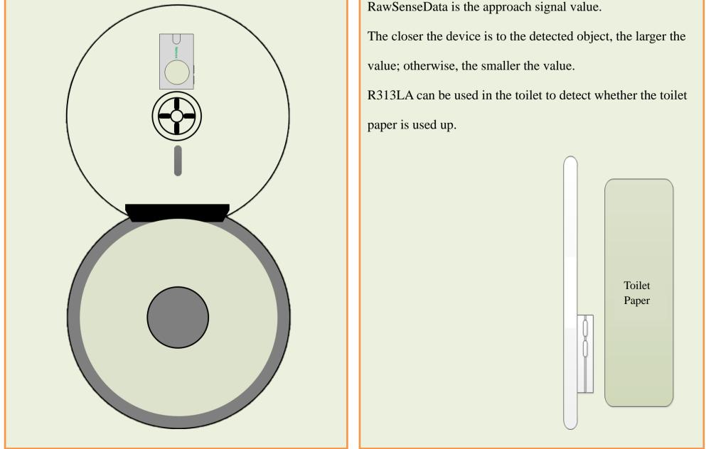
2. According to the situation of different paper boxes, choose the appropriate installation position.
