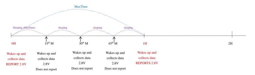
**Example#2** based on MinTime = 15 Minutes, MaxTime= 1 Hour, Reportable Change i.e. BatteryVoltageChange= 0.1V.
