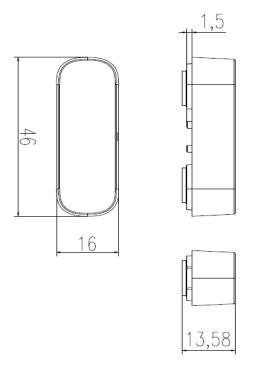
Water Leak Sensor (46mm x 16mm x 13.58mm)
