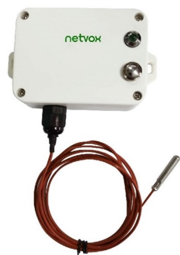
R718B120 - Round head probe -70° to 200°C
