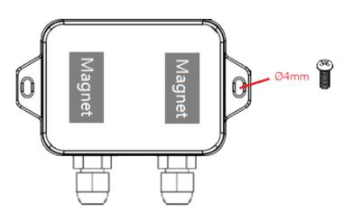
Screw hole diameter: Ø4mm
