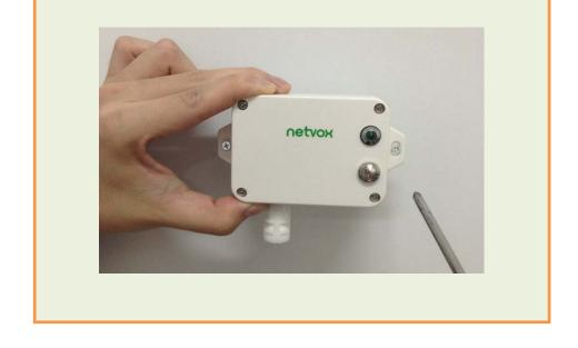
2. When Wireless Thermocouple Sensor is compared with the last reported values, the temperature change is exceeded 10°C (default), it will report values at the MinTime interval. If does not exceeded 10°C (default), it will report values at the MaxTime interval.
