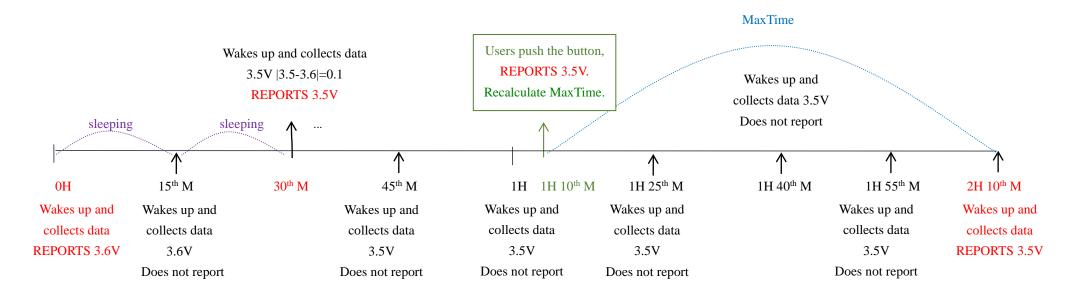
The device only wakes up and performs data sampling according to MinTime Interval. When it is sleeping, it does not collect data.
