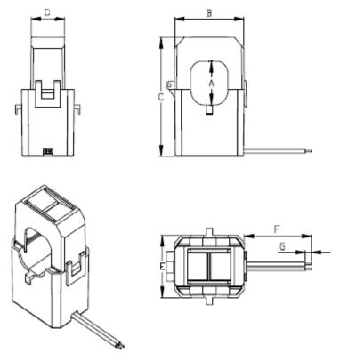
Figure 3 Clamp-on CT Dimension
