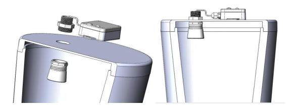
2. The container has no upper cover that can be opened. A circular hole with a diameter of about 45mm must be opened at the top of the container. A 32.4\*57.4\*3mm gasket is added between the ultrasonic probe and the bell mouth, as shown in the figure for reference.
