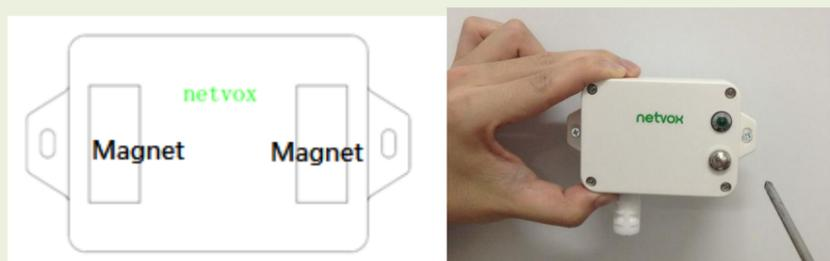
2. Peel the backings off the double-sided tapes on reed switch and magnet. Fix the reed switch and magnet on the door.
