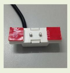
3. When the sensor probe detects the leak, the device will send an "alarm" message.
