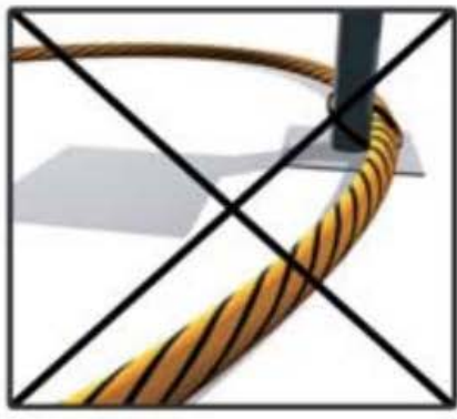
binding with metal (susceptible to interference)
