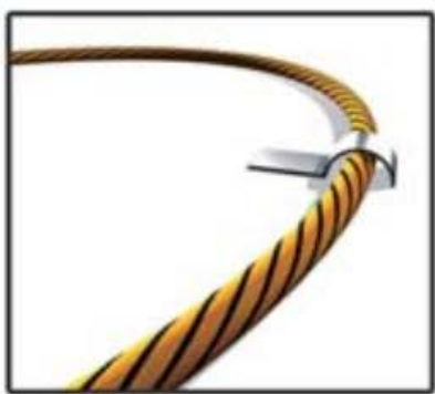
fixed by cable clips (recommend)
