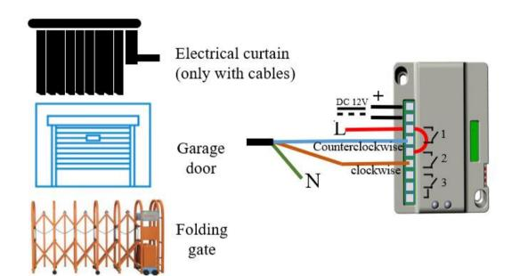
(1) Device type:electrical curtain, garage door, and folding gate(relay on: start operation; relay off: stop operation)
