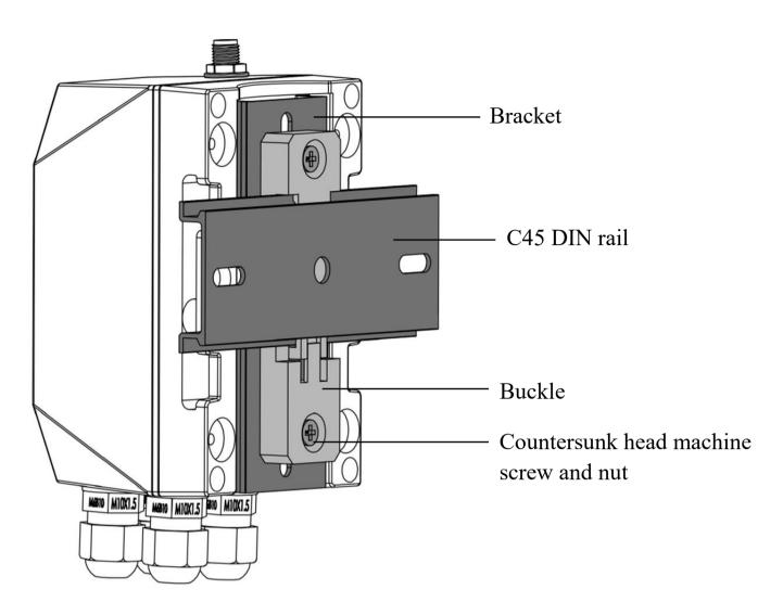
① Mount the rail buckle onto R900's bracket with countersunk head machine screws and nuts.
