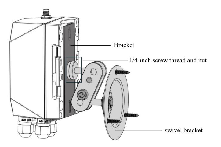
1 Insert a 1/4-inch screw thread into the hole of the bracket.
