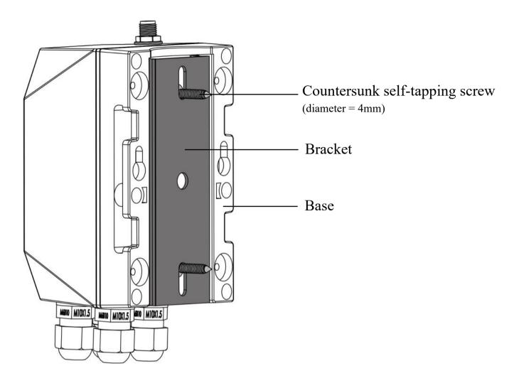
• Mount the bracket on a surface with 2 counter self-tapping screws.
