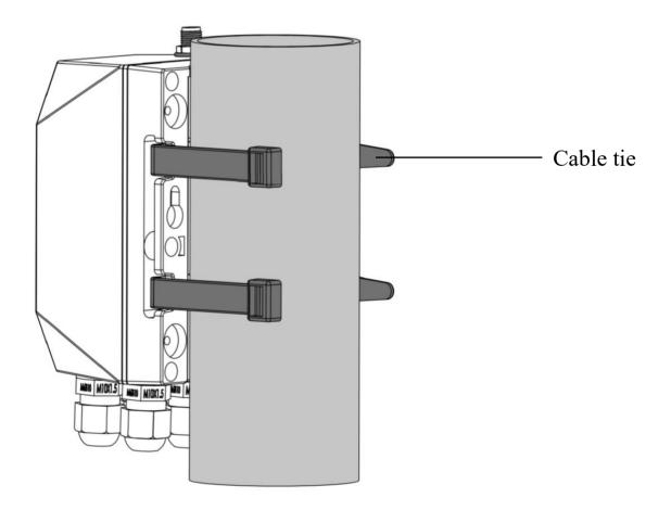
1 Insert cable ties through the holes of the base.
