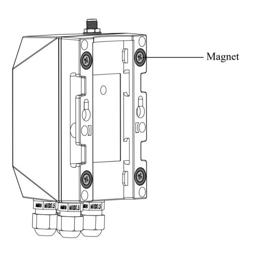
• Fix the R900 on a metal surface.
