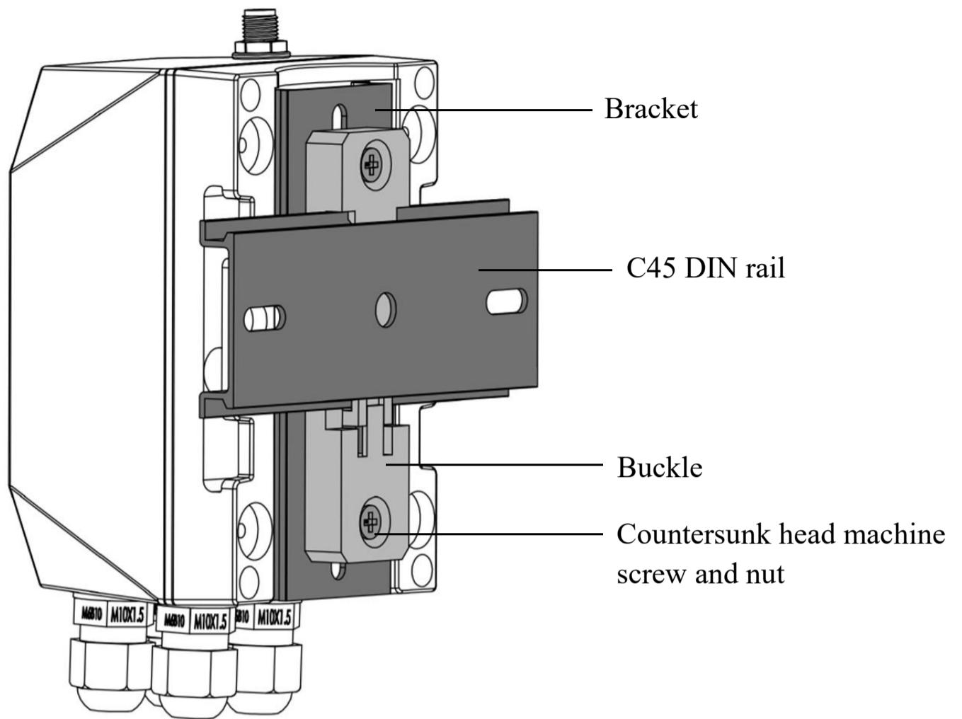
① Mount the rail buckle onto R900's bracket with countersunk head machine screws and nuts.
