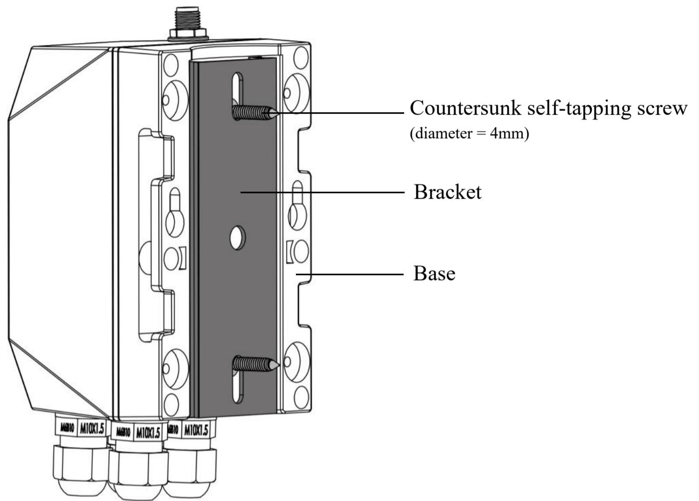
① Mount the bracket on a surface with 2 counter self-tapping screws.
