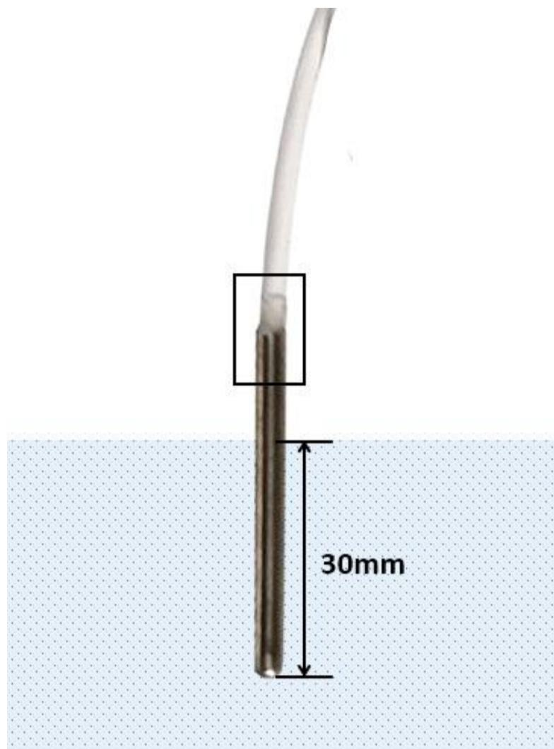
① The length of the stainless probe is 50mm. Please immerse it to a depth of 30mm.
