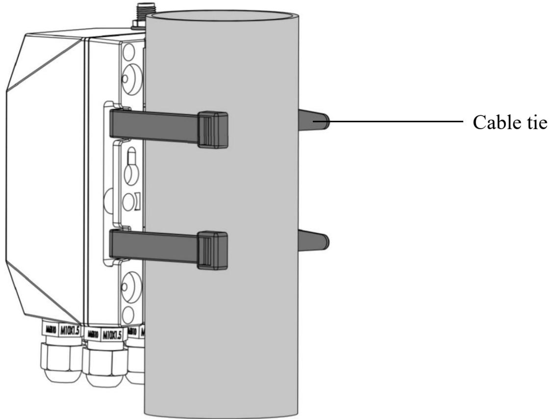
① Insert cable ties through the holes of the base.
