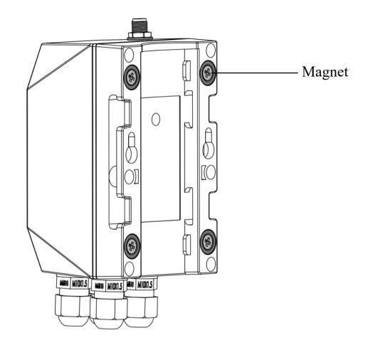
1 Fix the R900 on a metal surface.
