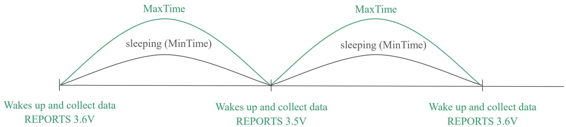
Note: Max Time = Min Time. Data will only be reported according to Max Time (Min Time) duration regardless Battery Voltage Change value.
