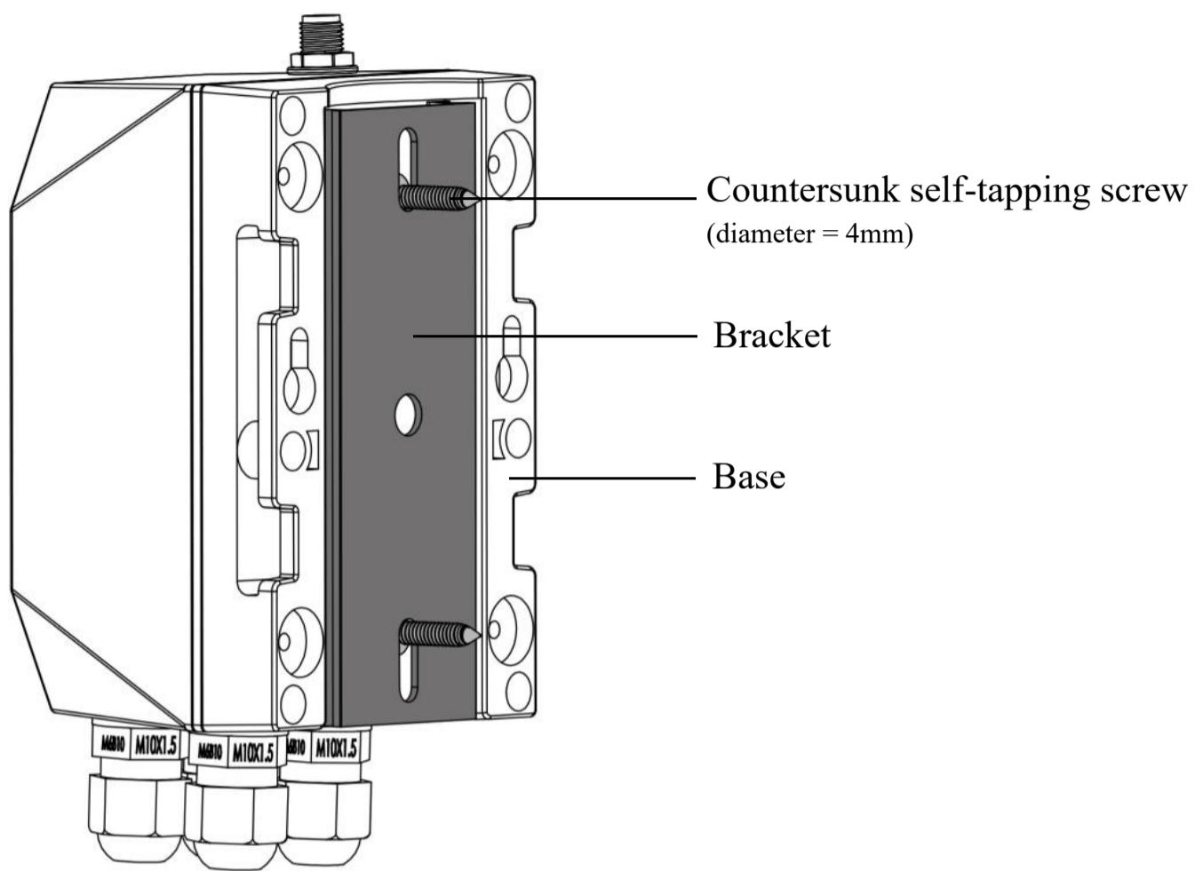
① Mount the bracket on a surface with 2 counter self-tapping screws.
