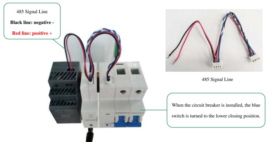
4. The wiring diagram of 12VDC power module, LoRa/LoRaWAN Radio Module, circuit breaker and load are as follows:
