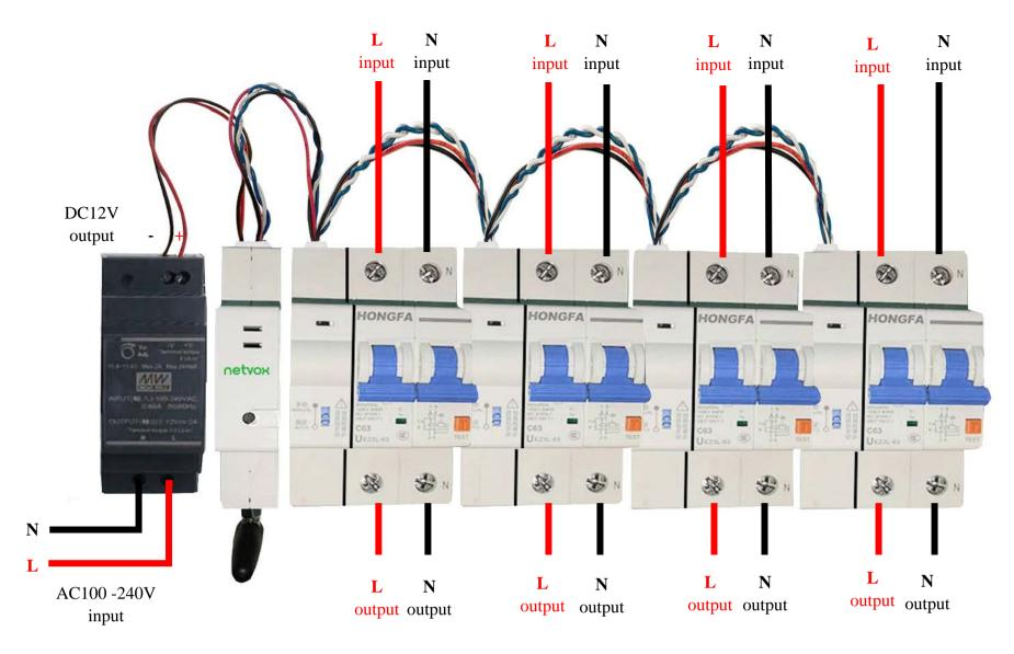
(b) Power Module + LoRa/LoRaWAN Radio Module + 1PNL\*4
