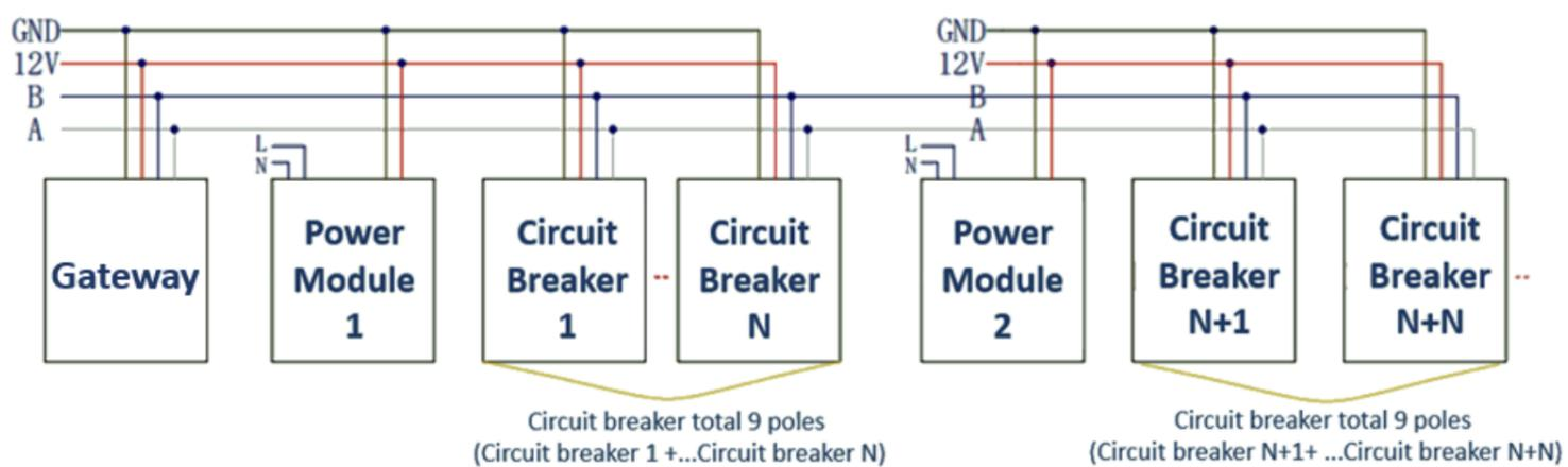
The output power of the power module is 24W, and the combined wiring diagram of the number of circuit breakers that can install the load is as follows:
