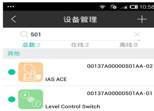
2. Select “Level Control Switch” to enter setting interface. In the setting interface, respectively, users can select the device to be bound with as shown below:
