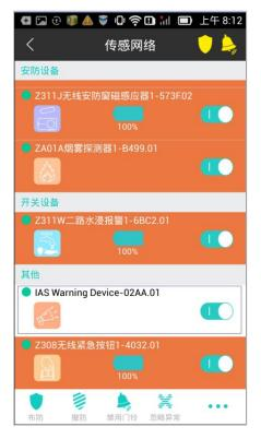
While alarm is on, users can press shortly the icon shown in below to stop warning. Long press the device icon at the control page, select "control" button to detail device interface. Select "Add to home page", to add device to present home page.
