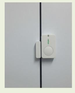
Places which are necessary to detect the opening and closing state
