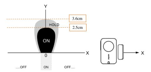
If the magnet moves along the Y axis relative to the sensor, it will cause repeated reports due to the magnetic field.
