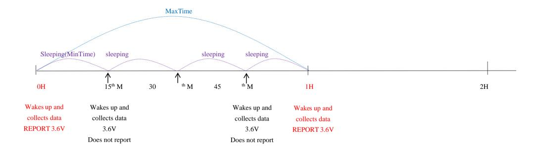
**Example#3** based on MinTime = 15 Minutes, MaxTime= 1 Hour, Reportable Change i.e. BatteryVoltageChange= 0.1V
