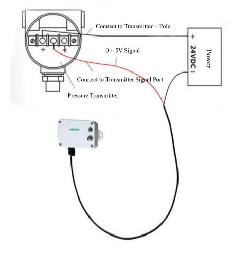
Figure 1 2-wire System Example Diagram (for wiring reference)
