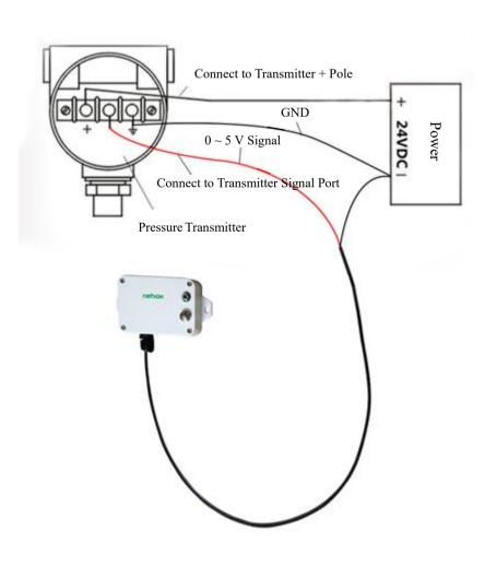
Figure 2 3-wire System Example Diagram (for wiring reference)
