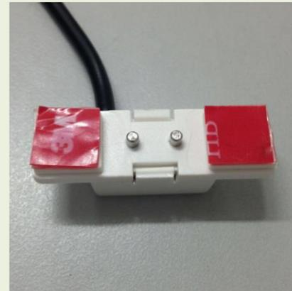
3. When the sensor probe detects the leak, the device will send an "alarm" message.
